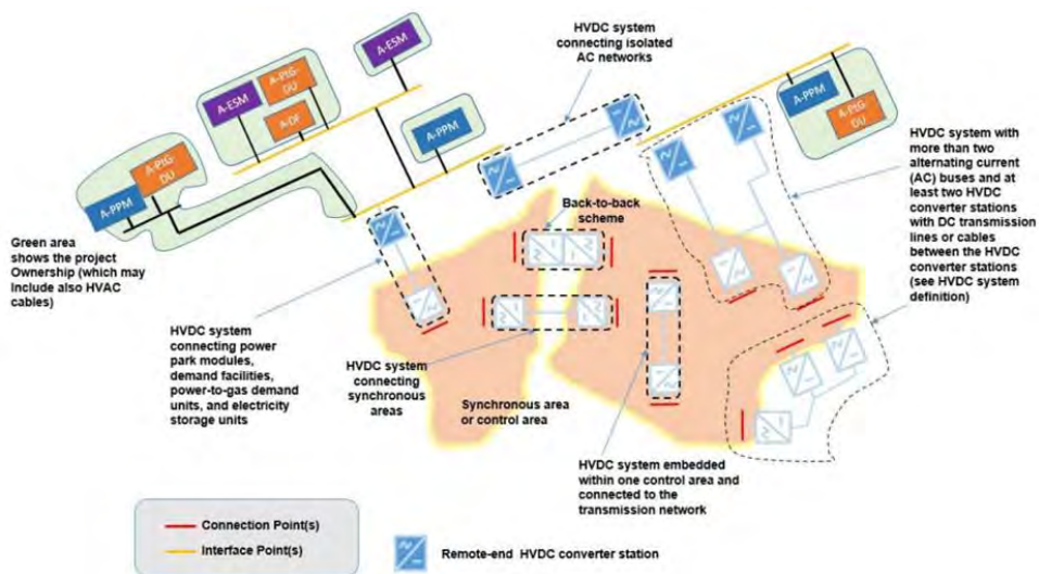
Figure 15 Explanation of NC HVDC 2.0 applicability and the relation to the definitions of the connection point and the interface point. (Source: Expert Group on Connection Requirements for Offshore Systems – Phase II (Proposal for the NC HVDC amendment), 10.11.20.
